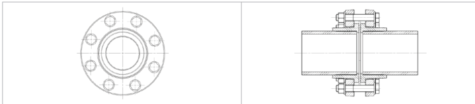
Flange with main axes (centered, crosswise)
