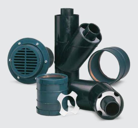
Fuseal Squared pipe is manufactured to ASTM F1412 requirements and all Fuseal Squared standard fittings are fabricated to DWV patterns utilizing butt-welding technology. Fabrication allows for precise production tolerances which provide for an optimal fit between the primary and containment fitting, as well as assuring standard connections to single wall Fuseal. The size range for pipe and fittings includes 11/2"×4" through 8"×12".
