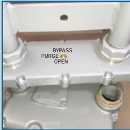
5. Turn the Co-Pilot to PURGE. Purge for one revolution of 1/2 ft. mark
