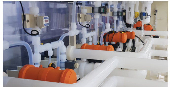
PVDF-HP components avoid corrosion in ultrapure water systems.
