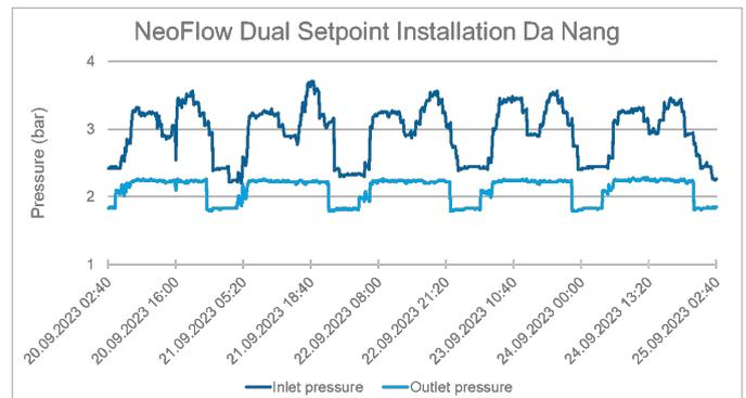
Pressure graph of the NeoFlow DN150 Dual Setpoint Valve at Cam Le, Da Nang
