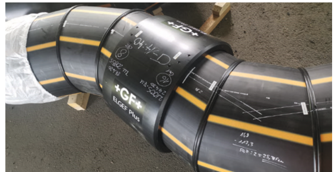
Pre-fabricated level modules: Segment elbows and ELGEF Plus coupler.
