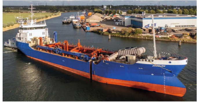
The HDPE ecoFIT pipes onboard the MS Zeeburg are part of the jet lines that are necessary for the mining process.
