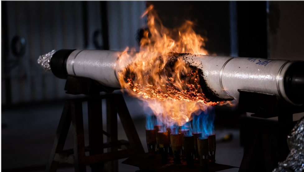
HEAT-FIT PE Fire Resistant test (IMO Res. A753 fire endurance L3 Code)
