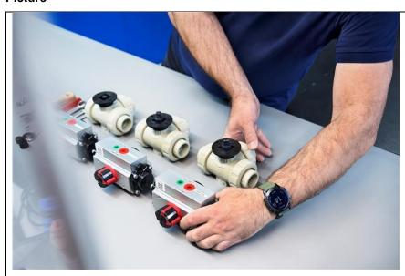
Actuator being mounted on a valve in valve automation center.
