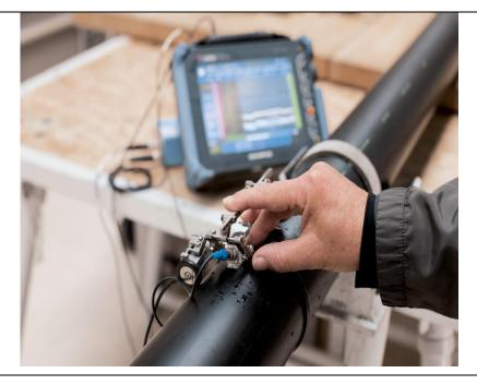
Ultrasonic Non-Destructive Testing (NDT) ensures leakage-free piping systems in data centers.
