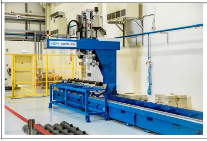
As part of the recent facility extension, GF Corys can now locally produce crucial piping components with the SWFM-630 Side Wall Fusion Machine by GF Piping Systems
