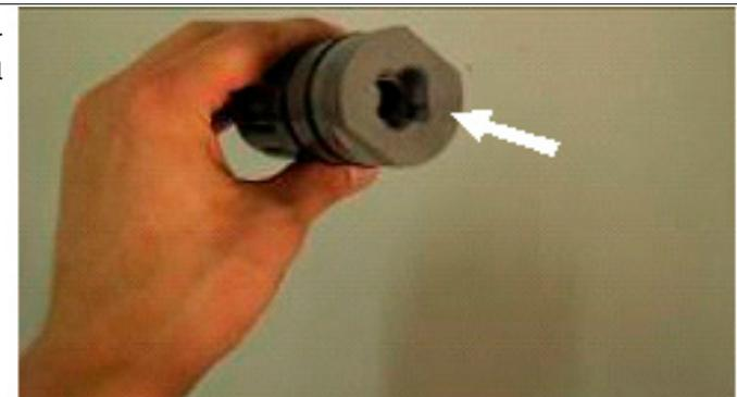
4. Check if the stem is flush with the bottom of the connecting element.
