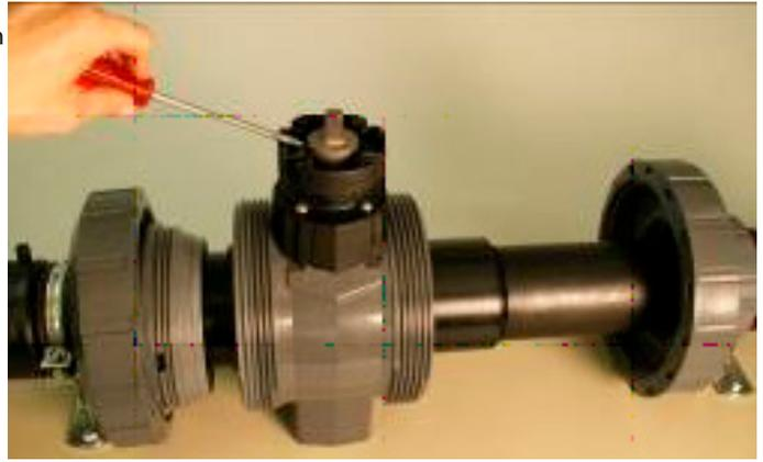
9. Move the protective housing aside. The ball valve is now accessible.
