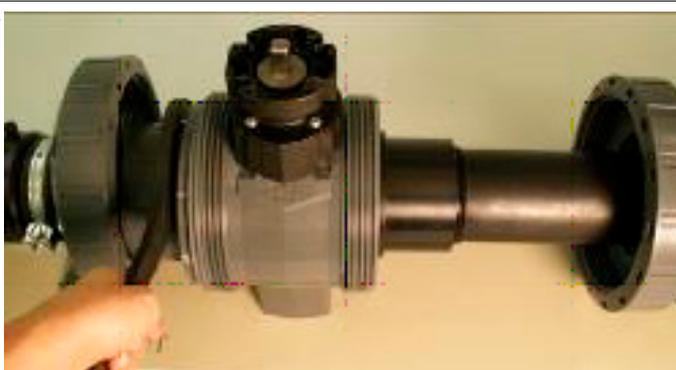
8. Remove the stem from the protective housing. A groove on the stem allows the use of a screw driver.
