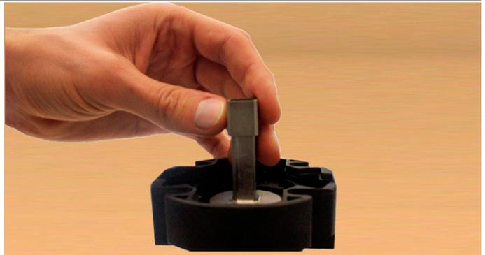
7. Mount the actuator with the adaptor interface on the connecting element.
