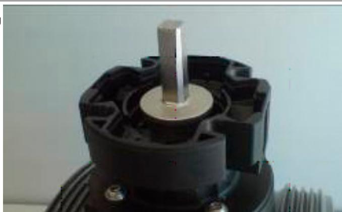
5. Screw the union bush (left-hand thread!) into the protective housing and tighten it. The use of a pin wrench (00 23 90) is recommended.
