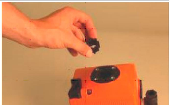
5. Mount the adaptor interface with four screws onto the actuator.
