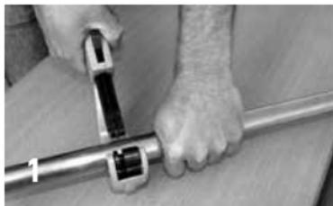
Cut the stainless steel or copper pipe with a commercial pipe cutter or a saw with fine teeth.
