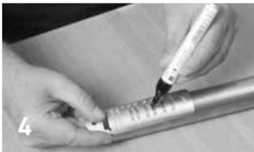
Mark the insert measure with the marking tool according to the pipe.
