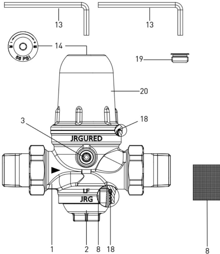
The plug **19** must be removed first with a Allen key 6 mm, before the pressure adjustment can be made.
