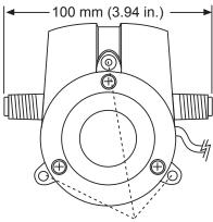
Mounting tabs for metric M3 or standard #6 screws on 68 mm (2.68 in.) bolt circle
