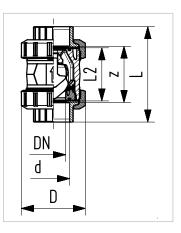
Type 561/562 with solvent cement spigots, metric
