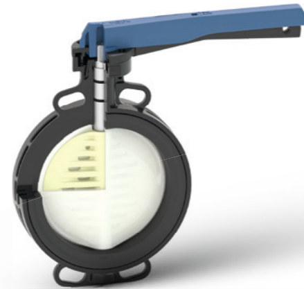
Figure 3: The low weight of the 565 results from a housing made of fiber reinforced polyamide and a polyvinylidene difluoride valve disc.
