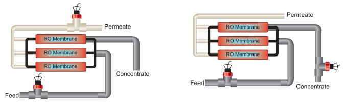
% Recovery A: (Permeate ÷ Feed) x 100 In the Setup menu, select the option that states % Recovery A, FEED: PERMEATE
