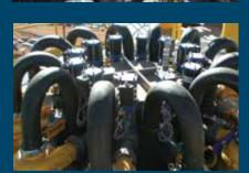
Cyclones are most commonly utilised in the classification of ore particles. A rotation of slurry inside the cyclone causes centrifugal force to move particles outwards. Larger mass particles migrate downward on the walls of the cyclone and discharged as underflow. Finer particles and water migrate upwards and discharge as overflow. GF Products are used for transport of ore
