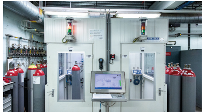
Leftover residue in gas storage cylinders and containers needs to be neutralized before they can be refilled.
