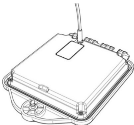
Figure 4.13 Charging the transmitter Li-Ion battery pack
