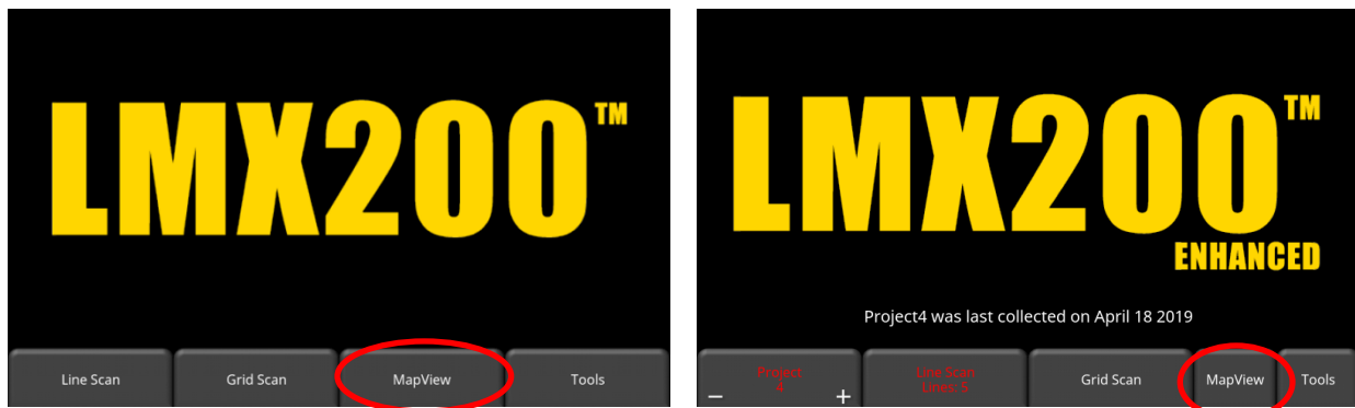
Figure 9-1: Accessing MapView from the main screen: a) LMX200 on left and b) LMX200 Enhanced on right
