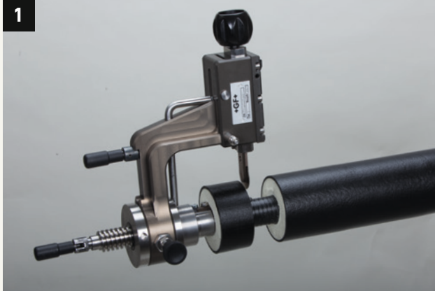
1 The GF foam removal tool helps to remove the foam and peel the pipe efficiently.
